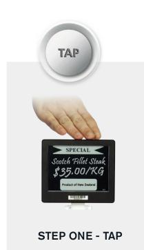
Tap e.Label for the product chosen. This triggers a signal for the product's PLU to be transmitted to the scale.
